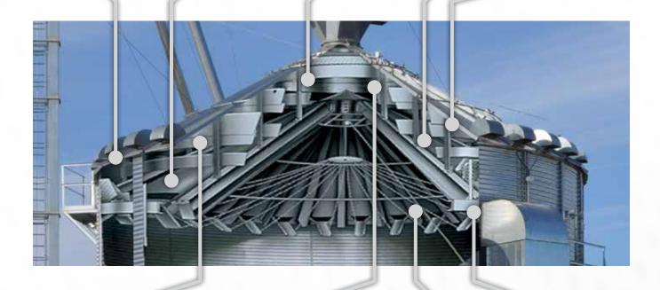
Leveling bands maintain even grain depth. Industrial rotary switches mounted in the bin wall and roof indicate drying and storage chamber levels. This allows the AutoFlow's automatic operation and will stop either model if the storage chamber becomes full. On a Batch TopDry, a horn signals when the drying chamber is full.
