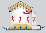
**Step 2.** Outside air from the cooling fan captures heat from previously dried grain and that heat and aeration air is used to help dry the next batch.
